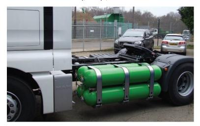
"Too many people get hung-up on the substitution rate. You can get 60-70%, but if that's at 15-20% efficiency slip [CNG litres versus pure diesel litres per km], then the real cost per mile is hit hard. With our system, the overall efficiency slip is just 4-8%."
